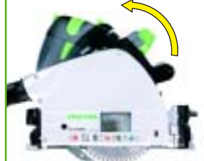
Step 3: close Fast Fix lever.
