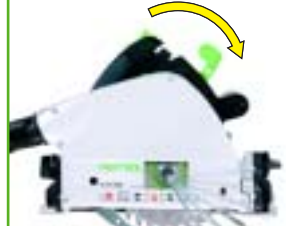
Step 2: Unscrew the Allen screw, change the saw blade and drive the Allen screw back in.
