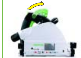
Step 1: open the Fast Fix lever.
