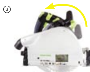
③ Insert the new blade, tighten the bolt, close the FastFix lever and move the machine upwards. Done.
