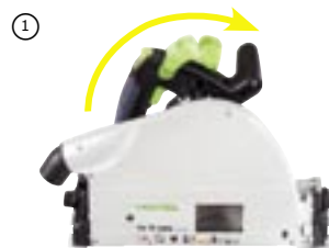
① Open the FastFix lever, press the machine down as if you are plunge-cutting until you hear it engage. The spindle stop is activated.
